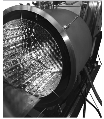
Opened chamber of the UNIVEX 1000 S with temperature controllable shrouds and substrate tray
