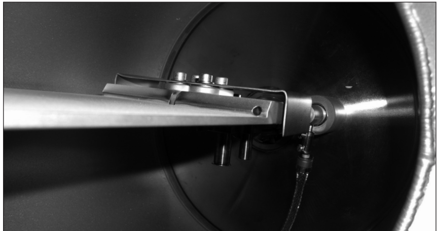
Insulated substrate fork with RF bias connection
