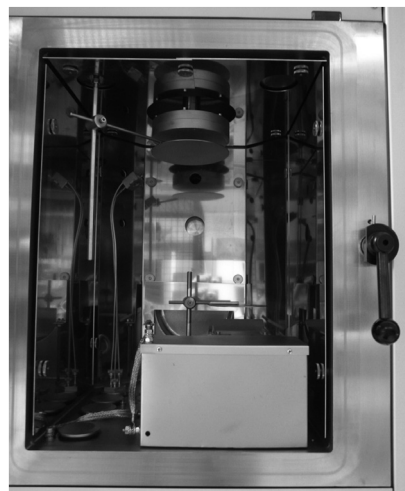
Rotating and water-cooled substrate table
