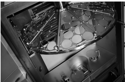
Chamber bottom: electron beam evaporator, thermal evaporator, ion source Chamber top: rotating substrate dome with turnover device
