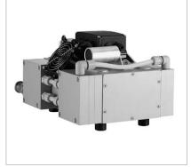
in the lower pressure range a higher pumping speed compared to conventional diaphragm pumps. At the same time they are capable of attaining ultimate pressures below 2 mbar (1.5 Torr) and are thus very well suited as backing pumps for turbomolecular pumps. Owing to their compact design they are also suited for installation
